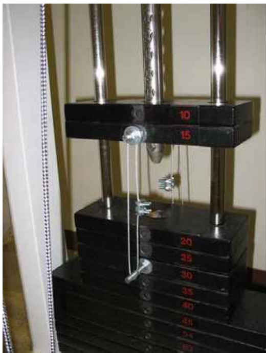
Figure 12: Mechanism with loops for adding weights
